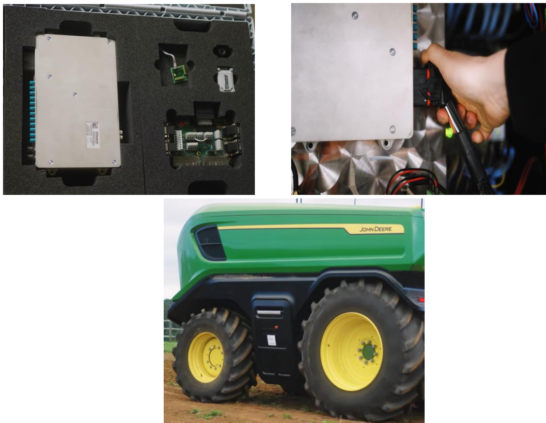
Figure 57: TTTech Hardware build in the tractor
