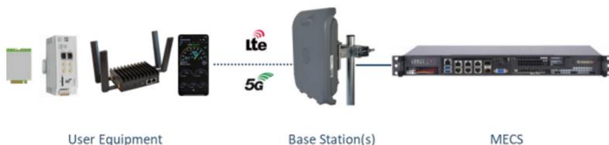
Figure 61: MECsware campusXG network with Application Server
