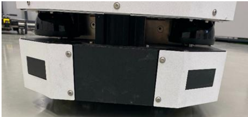
Figure 57. Photo of the laser scanners in the AGV
