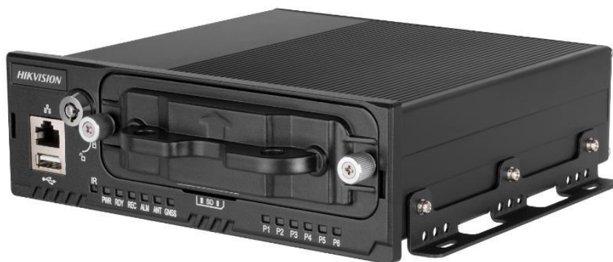
Figure 183. EUROGATE NVR connected to the IPTV cameras of the pilot.
