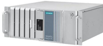
Figure 70. Pilot 1.3 Device compatible with Siemens Industrial Edge – SIMATIC IPC 547G
