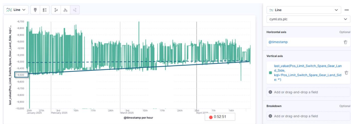
Figure 173. 200mm trolley wire rope elongation obtained by reviewing the spare gear limit switch position stored in the SL1520.3 register of the PLC of the STS crane 04.
