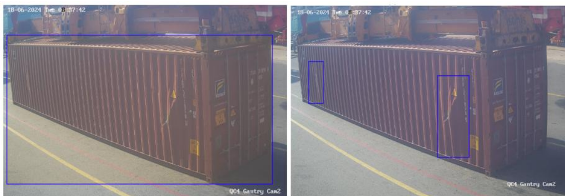
Figure 187: Sample of labelled images from (a) the container and (b) the damage datasets
