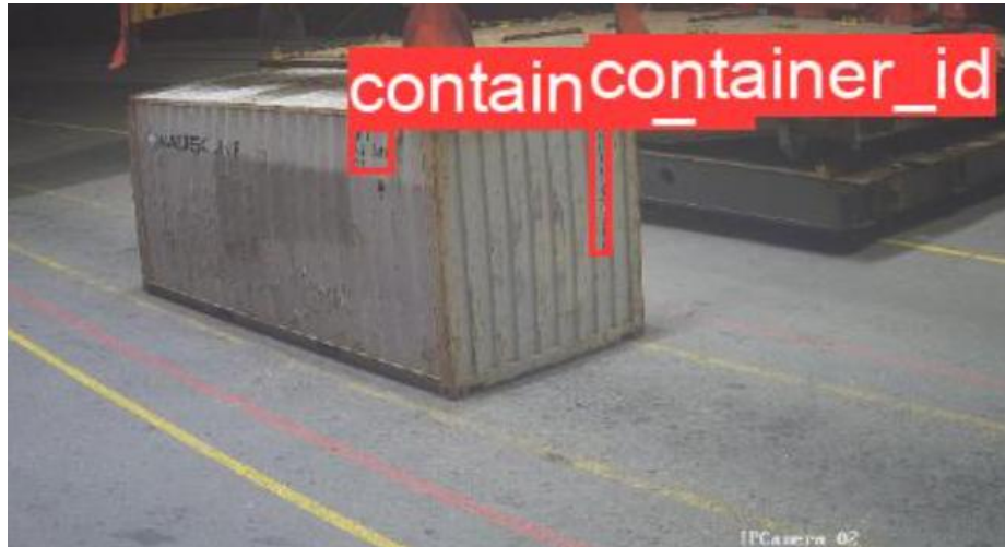
Figure 186. A sample labelled image with both horizontal and vertical container ID.
