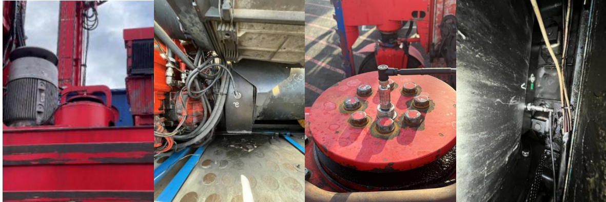
Figure 163. Pilot 4 Different sensors installed in the Straddle carriers under test in the project.
